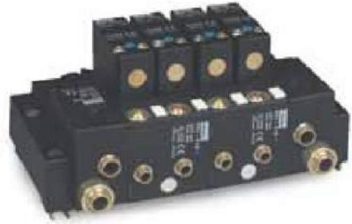
Poppet valve, not suitable for use with Soft or Slow start Valves. When pressure is applied, the double solenoid interface takes a pre-determined position (non activated). In the absence of electrical signal, output 2 (yellow indicator) is activated, output 4 (red indicator) is non activated. Double solenoid version is delivered as standard with Non locking flush override.
